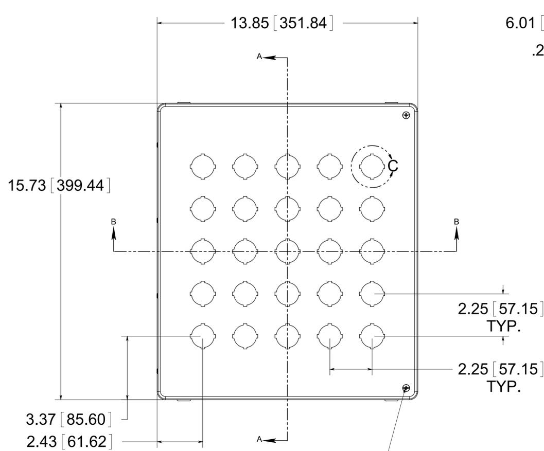
(2) EACH #10-32 BRASS INSERTS AND STAINLESS STEEL CAPTIVE COVER SCREWS WITH RETAINING O-RING
