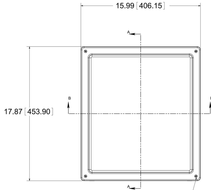
(4) EACH #10-32 BRASS INSERTS AND STAINLESS STEEL CAPTIVE COVER SCREWS WITH RETAINING O-RING
